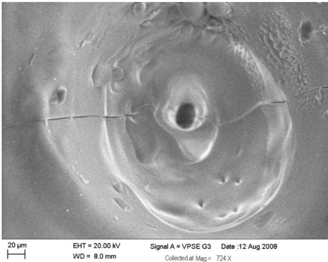
Laser drilled defect 5  $\mu\text{m}$
